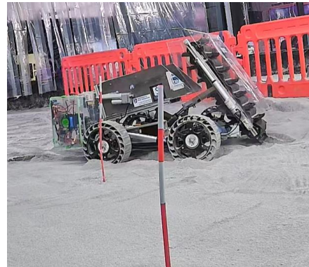
Fig. 1: Lunabotics excavator with stuck back wheel
